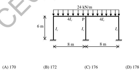
Q.34 A prismatic beam (as shown below) has plastic moment capacity of  $M_p$ , then the collapse load P of the beam is
