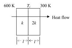
The interface temperature  $T_i$  (in K) of the composite wall is \_\_\_\_\_
